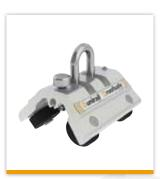
**Attachment carriage** – enables the user to connect to the system and enjoy complete hands-free movement along the rail. It features a stainless steel parking lock for work positioning tasks and hard anodised aluminium wheels. A stainless steel shackle enables connection of a karabiner hook and pivots to enable best functionality at any angle of take off. Min strength 15kN (3300lbs)
