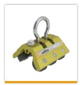
WT UniRail carriage – the carriage is part of the Unirail system. It provides a mobile attachment point for users to connect to. One user per carriage. Use only on straight systems. Minimum strength 22kN (5,000lbs)
