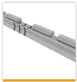
Flexirail Insert – to allow a continuous system to be fitted where two adjoining sections of rail need to be mounted to parts of the structure which can move independently of each other. In a UniRail commercial marine system.
